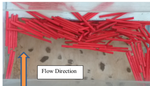
Figure 4. Top view of wood accumulation at the model bridge
